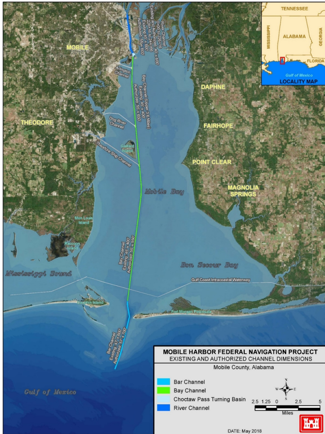
Figure 1. Mobile Harbor Federal Navigation Project Limits and Dimensions
