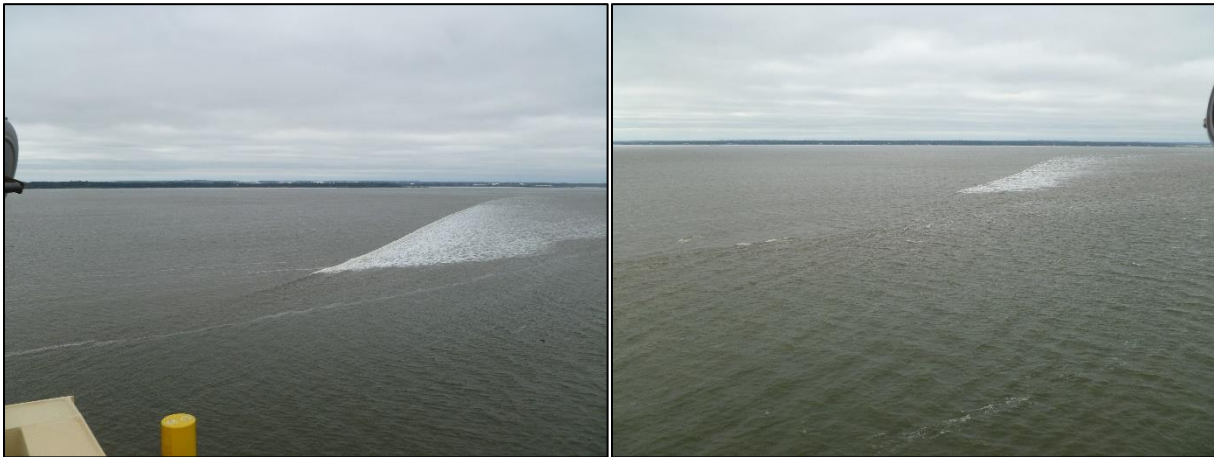
Figure 21: Observed breaking of vessel generated wake. Photos taken looking west from an outbound tanker on 09 November 2017. Vessel dimension: L = 244 m, B = 42m. Vessel draft on the date of picture was 8.5m. Left picture was 7 km and right picture 4km north of instrumentation stations.
