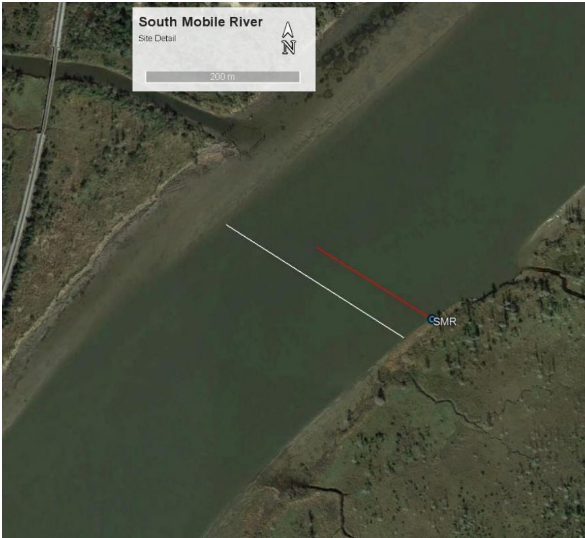
Figure 23. South Mobile River (SMR) site detail. The location of the site instrumentation is shown with a blue circle, the location of the boat-based ADCP transect is shown with a white line, and the extent of the horizontally-averaged HADCP beam is shown in red.
