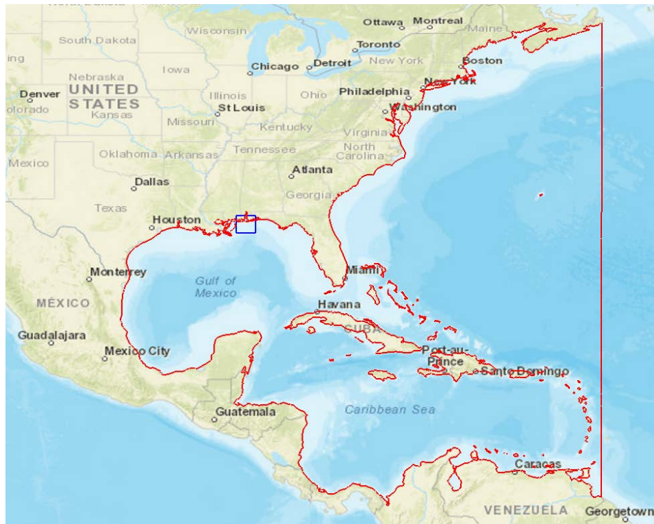
Figure 3. ADCIRC domain boundary, Red, and STWAVE boundary, Blue.
