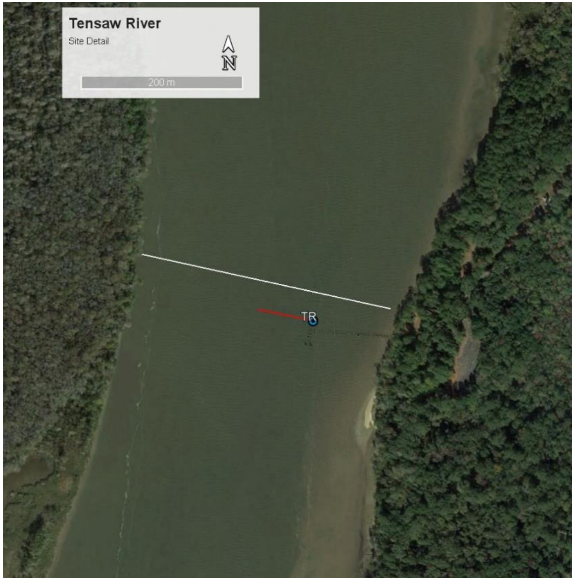
Figure 13. Tensaw River (TR) site detail. The location of the site instrumentation is shown with a blue circle, the location of the boat-based ADCP transect is shown with a white line, and the extent of the horizontally averaged HADCP beam is shown in red.
