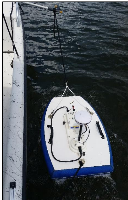
Figure 3: Sontek M9 Acoustic Doppler Current Profiler Field Deployment Configuration.
