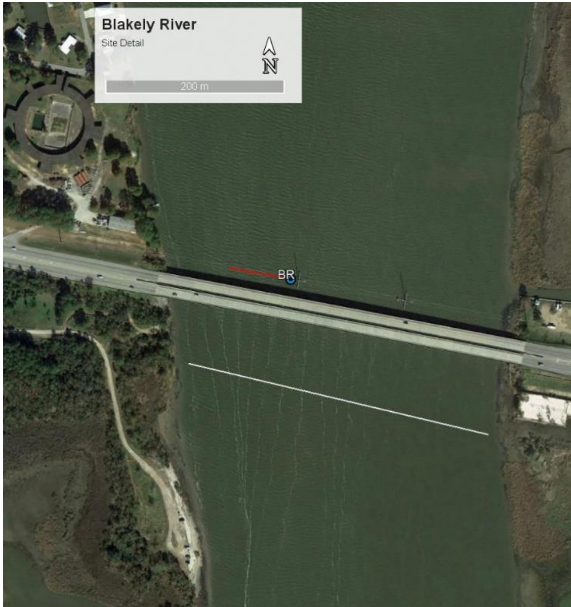
Figure 54. Blakely River (BR) site detail. The location of the site instrumentation is shown with a blue circle, the location of the boat-based ADCP transect is shown with a white line, and the extent of the horizontally average HADCP beam is shown in red.
