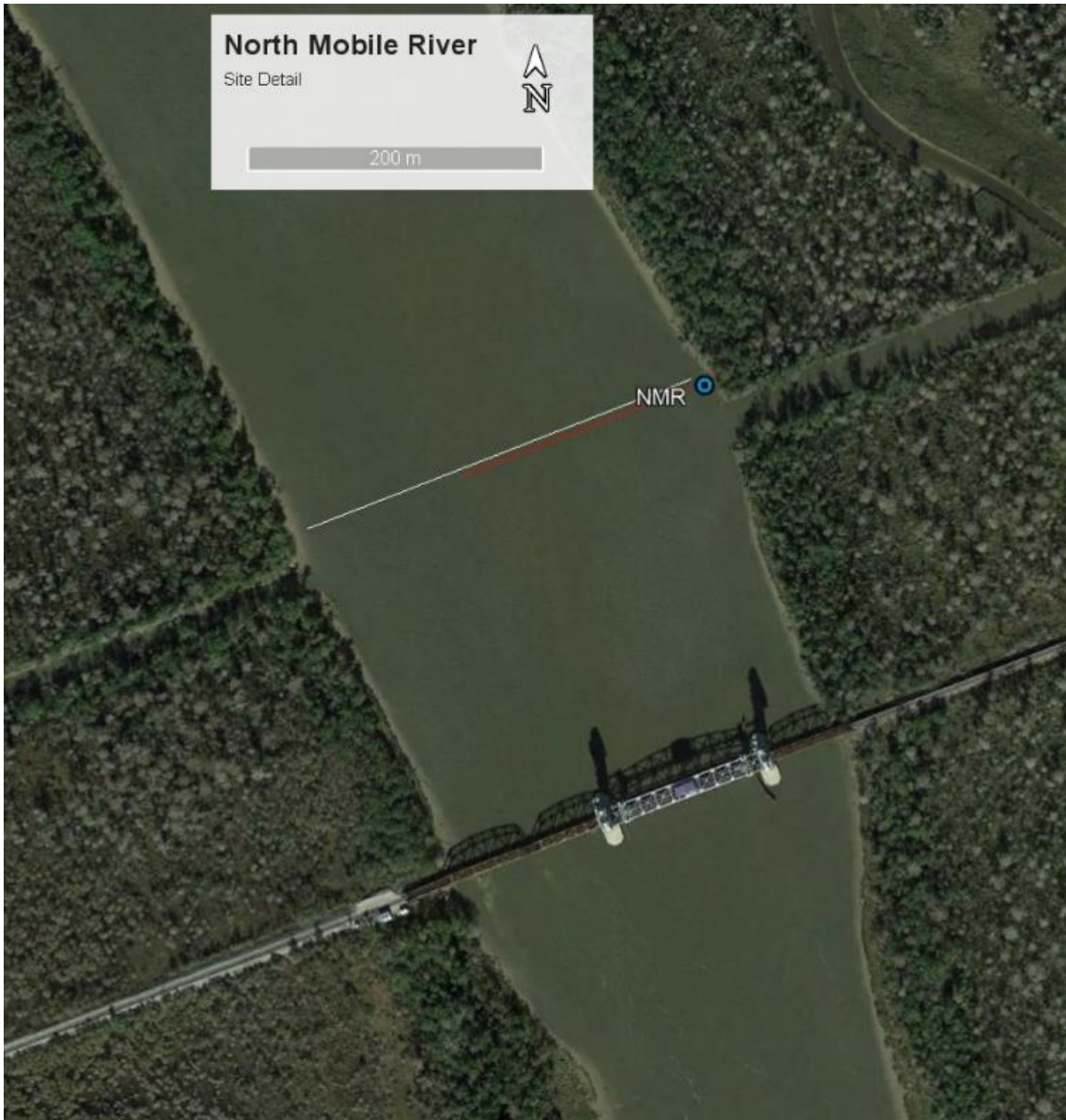
Figure 3. North Mobile River site detail. The location of the site instrumentation is shown with a blue circle, the location of the boat-based ADCP transect is shown with a white line, and the extent of the horizontally averaged HADCP beam is shown in red.
