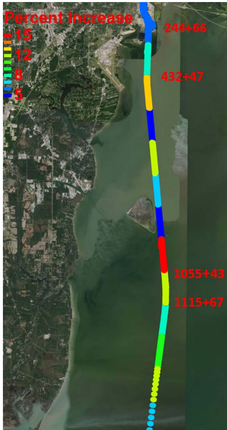
Figure 109. Simulated increases in annual shoaling vary from 5 to 15 % along channel with-Project depths. Four channel stations are shown in red to the east side of the channel.
