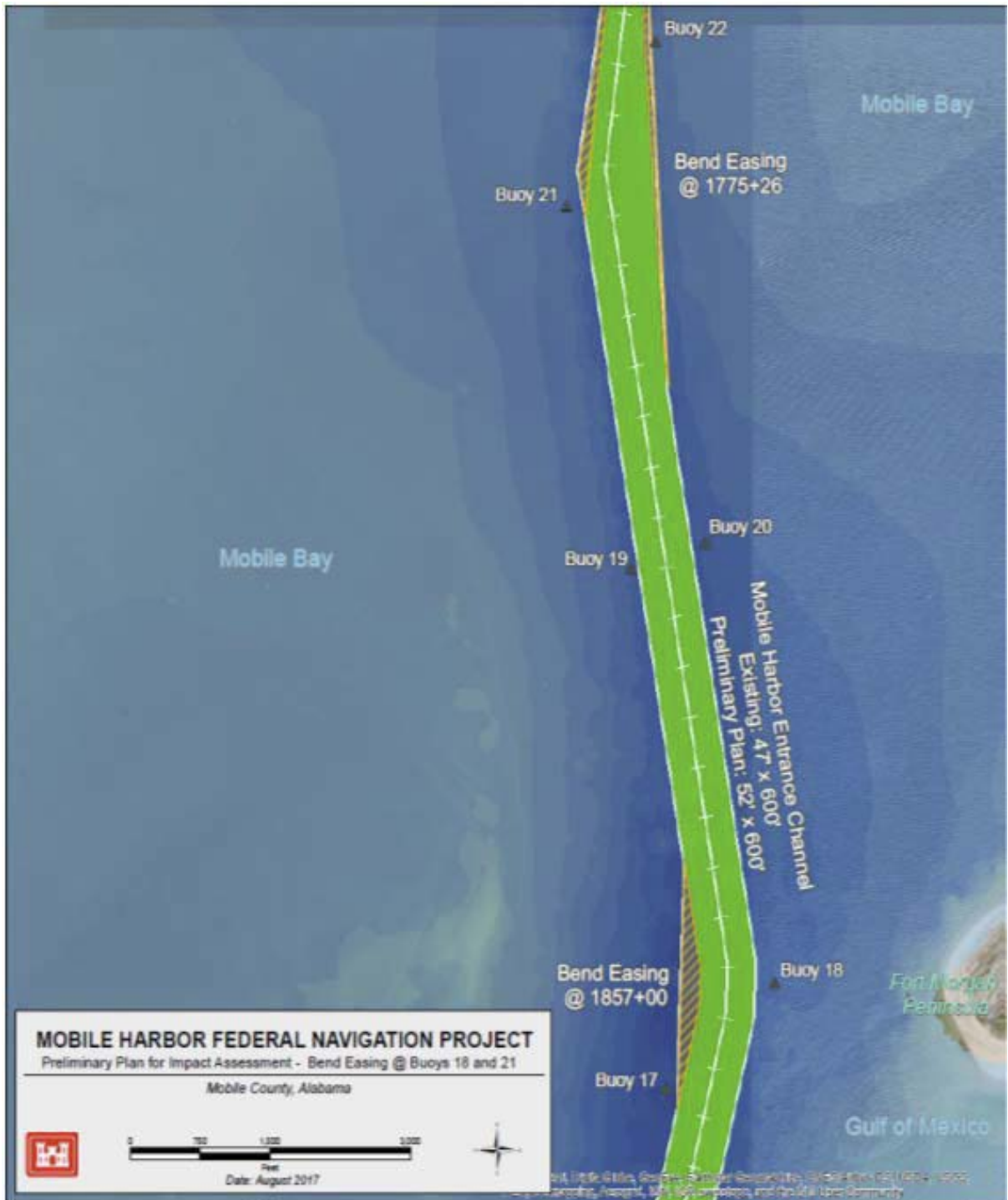
Figure 42. Bend Easing Design at the Mobile Bay Entrance
