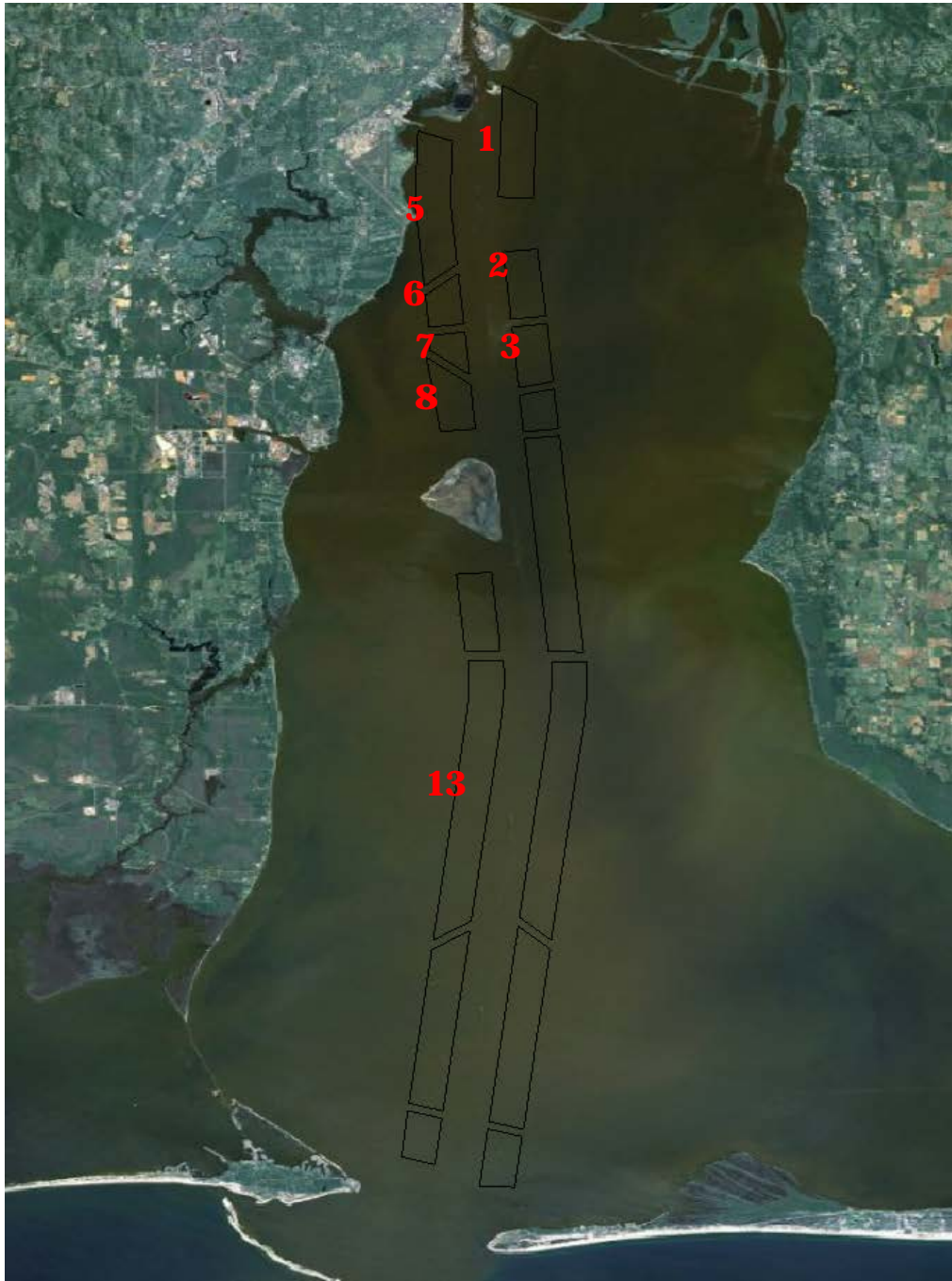
Figure 100. Placement Areas (black quadrilaterals) along the navigation channel. Number of Placement Area in red.
